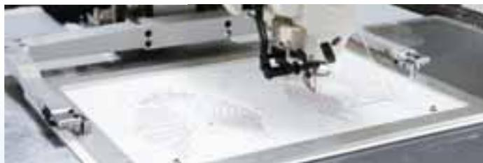
The machine performs various kinds of stitching, making the most out of its wider sewing area in various sewing applications such as attaching handles to bags and pouches, attaching belts, sewing many small parts at a time, attaching parts to shoes and sports shoes (one pair of shoes) and sewing air bags.
