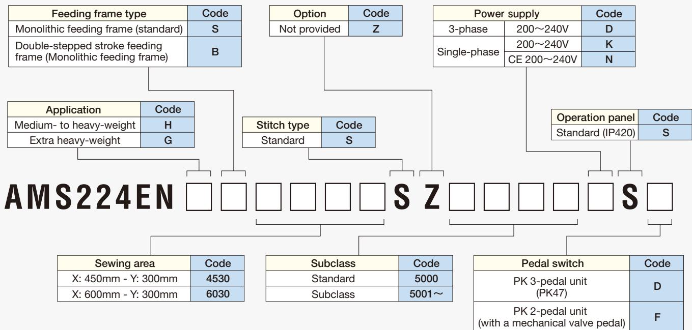
★ "D" (PK 3-pedal unit) should be selected for the feeding frame type with the double-stepped stroke feeding frame (B).
