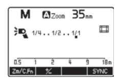
into 8 grades, each has maximum 3 grades for fine adjustment, with grade 0.3EV, 0.4EV as adjustment increment, totally 29-grade fine adjustment. After the flash output set, half press the shutter release button, the screen will display the aperture value and flash effective range.
