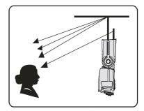
If the wall or ceiling is too far, the bounce flash may be too weak to get enough exposure. The wall or ceiling should be even and white in order to get efficient reflection; if the reflection surface is not white, color cast may appear in photo.
