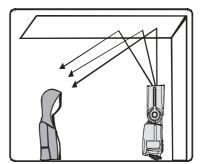
produce a highlighted point on the eyes of the subject and thus make the eyes charming (catching light). This function can reach optimal effect when the flasher head is up 90°.
