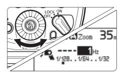
NOTE: When in low battery, the charging speed of speedlite will be slow, which may cause the leakage of the stroboscopic flash. In this situation, please reduce the flash frequency or change new battery.
