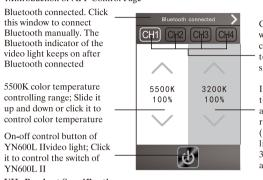
Channel switching window: Select more channel (8 channels in total) by clicking it or sliding it leftwards
