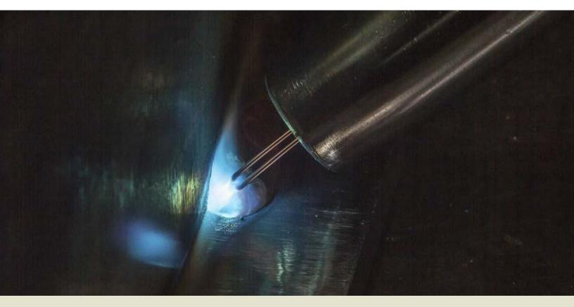
The HyperFill<sup>®</sup> twin-wire MIG solution was developed to revolutionize heavy fabrication productivity. Designed for semiautomatic and robotic applications, HyperFill redefines high deposition welding – allowing you to make larger welds, faster and more easily. With its innovative twin-wire design, HyperFill allows for deposition rates above 18 lbs/hr (24+ lbs/hr robotically ) without compromising weld quality or operator ease-of-use.
