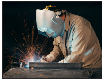
Conventional CV short circuit transfer using carbon dioxide (CO 2 ) and 0.045 in. solid wire.
