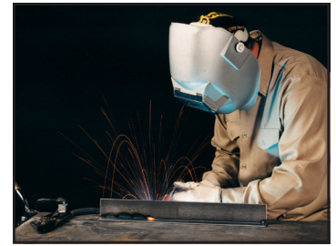
STT using CO 2 and 0.045 in. solid wire. (Note reduced spatter and fume).
