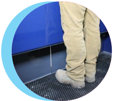
Foot indentation to allow operative to work with correct body posture.
